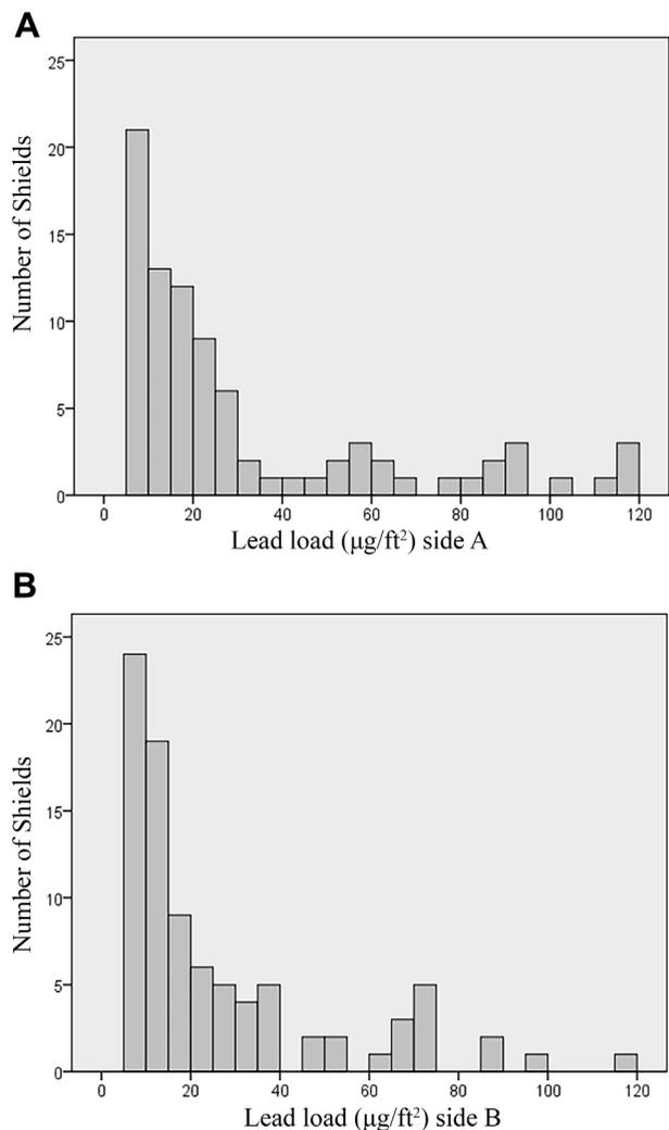
**Fig 2.** Distribution of detectable surface lead dust from shield side facing the wearer (A, inner) and away from the wearer (B, outer). Distribution truncated at 120. Seven shields had higher lead levels on the inner surface (152, 196, 219, 378, 840, 873, 998  $\mu\text{g}/\text{ft}^2$ ) and five shields had higher lead levels on outer surface (125, 159, 230, 347, 703  $\mu\text{g}/\text{ft}^2$ ).
